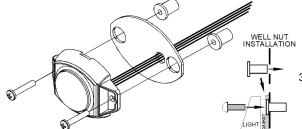
Push the well nuts through the holes until the lip rests on the surface.
